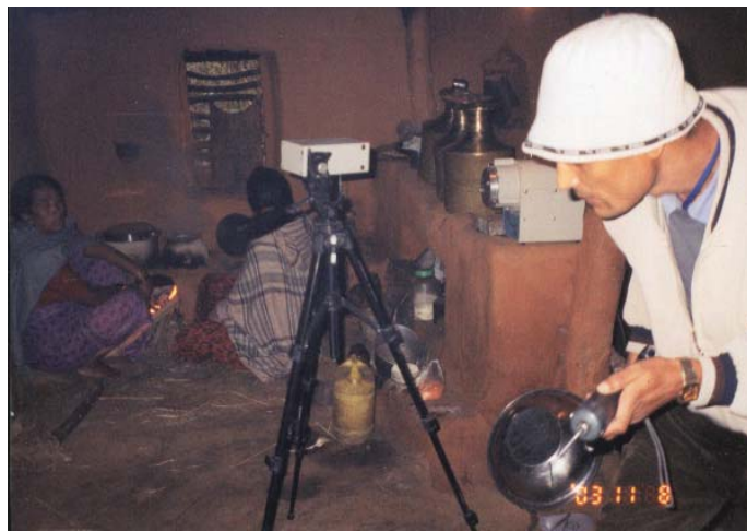
Kitchen PM_{10} Monitoring by LD-1, HVS and CO by Gas Analyzer; Katunje VDC, Bhaktapur
