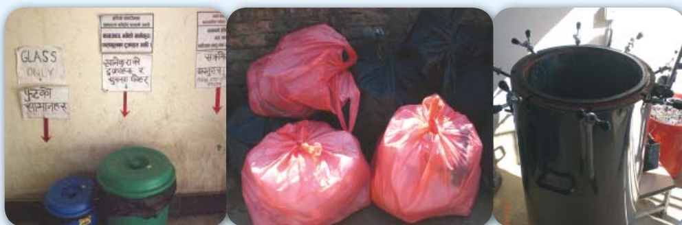
Figure 77: Hospital waste management system i.e. Source separation, collection & transfer appropriately and separately and treat with autoclave
