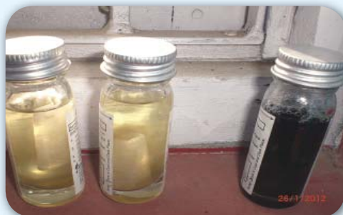
Figure 5: Drinking Water Sampling Shows Coliform Contamination
