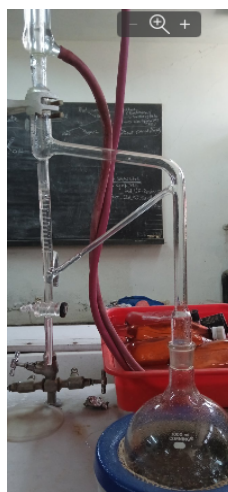
Figure 14. Extraction using Clevenger apparatus
