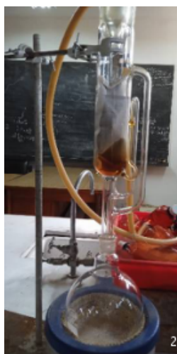
Figure 13. Extraction using Soxhlet extractor
